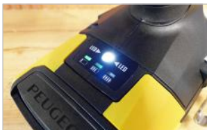
Eclairage LED de la zone de travail LED light of the working area
