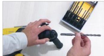
Mandrin SDS+ SDS+ chuck
