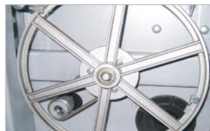
2 Volants fonte d'aluminium 200 mm 2x 200 mm cast aluminium wheels
