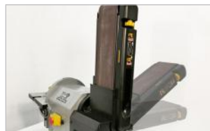
Bras inclinable de 0 à 90° 0 to 90° sanding belt tilt adjustment
