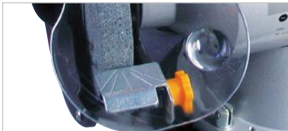
Support d'outil rainuré Grooved tool support
