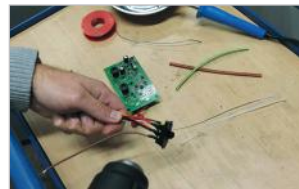
Pose de gaine thermo-retractable Heat-shrink tubing installation
